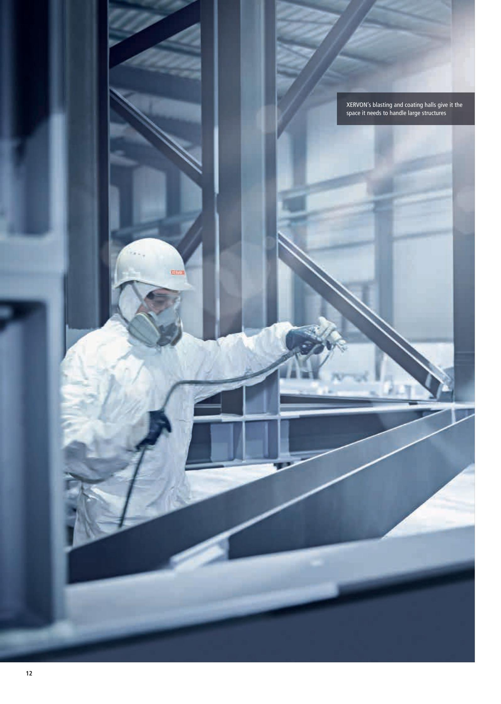
A worker in a white protective suit and helmet is using a spray gun to apply a coating to a large metal structure in a factory. The worker is wearing a white hard hat with a logo, a white protective suit, and a respirator mask. The background shows a large industrial facility with a complex steel framework.
